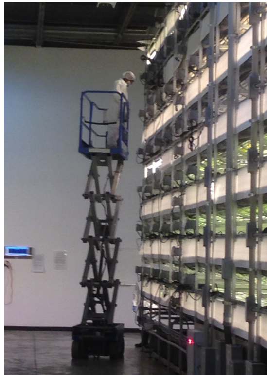
Fig. 3. A scissors lift is used to access crops on upper levels in a commercial plant factory.
